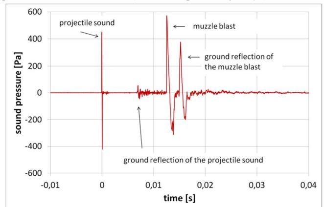
Figure 1 Pressure time history of the shooting sound projectile sound and muzzle blast at 10 m distance, 2 m height and at  $10^\circ$  re. line of fire
