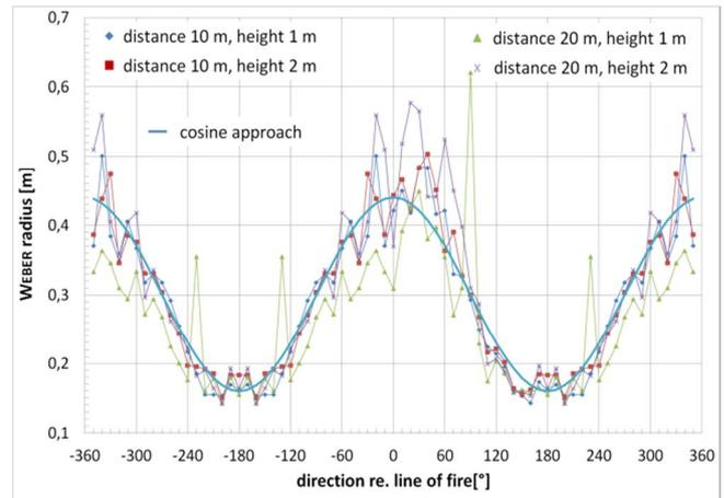
Figure 3 WEBER radius versus direction re. line of fire at four measuring positions and an optimized Cosine-fit  $R_{w0} = 0,3 \text{ m}$ ,  $e_w = 0,45$
