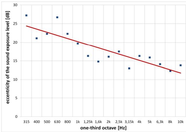
Figure 2 Difference of the one-third octave sound exposure level at 0° and 180°, distance 20 m, height 1 m
